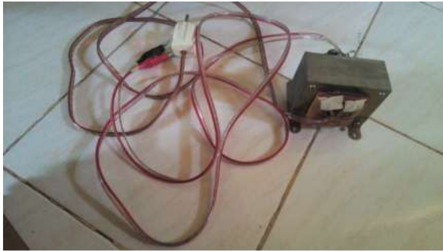
Gambar 2.5 Charger Akumulator (Aki)
