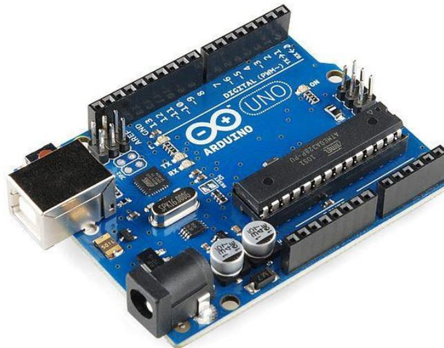
**Gambar 2.7** *Microcontroller* Arduino Uno (Arief, 2014)
