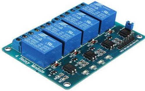
Gambar 3. Module Relay
